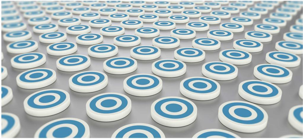
The tablets produced with Exentis' 3D technology are special because their active ingredient delivery profile can be freely adjusted in the human body. Image credit: Exentis
