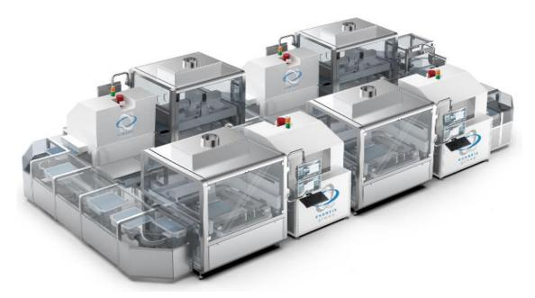
Modular Exentis Pharma production system for large-scale manufacturing of tablets with a freely adjustable release profile of active pharmaceutical ingredients in the human body, with up to three active ingredients on one tablet. Annual production capacity of up to 200 million tablets per system.
