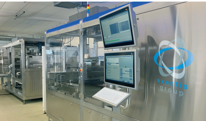
Exentis Pharma production systems for the manufacturing of innovative tablets with a freely adjustable release profile of the active pharmaceutical ingredients in the human body
